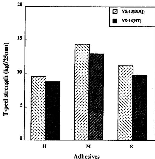
Fig. 8 T-peel strength of steel sheets for adhesives H, M and S. (YS : Yield strength of steel sheets (kg/mm<sup>2</sup>))
