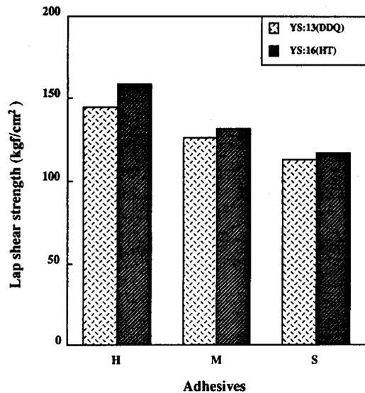
Fig. 7 Lap shear strength of steel sheets for adhesives H, M and S. (YS: Yield strength of steel sheets(kg/mm<sup>2</sup>))
