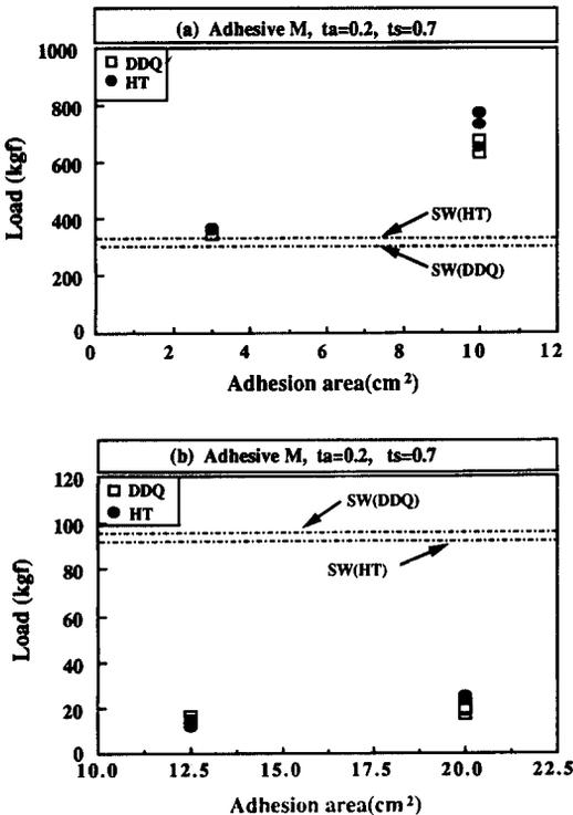
Fig. 11 Adhesion strength versus spot welding strength. (Nugget dia. for spot weld : 3.3mm)
