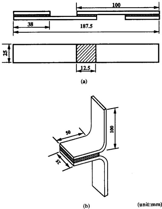
Fig. 1 Schematic diagram of specimen for bonding strength test.
