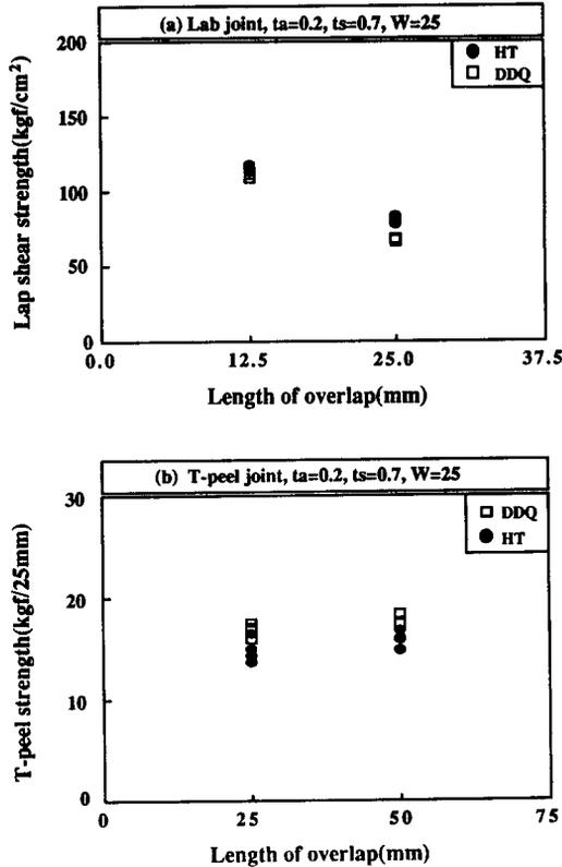
Fig. 9 The effect of joint length upon the lap shear strength and T-peel strength for epoxy(M) adhesive bonding steel sheets.
