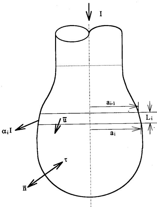
Fig. 2 Maxwell stress acting on the molten drop
