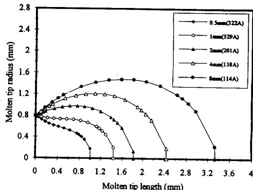
Fig. 4 Molten tip shapes for various initial volumes
