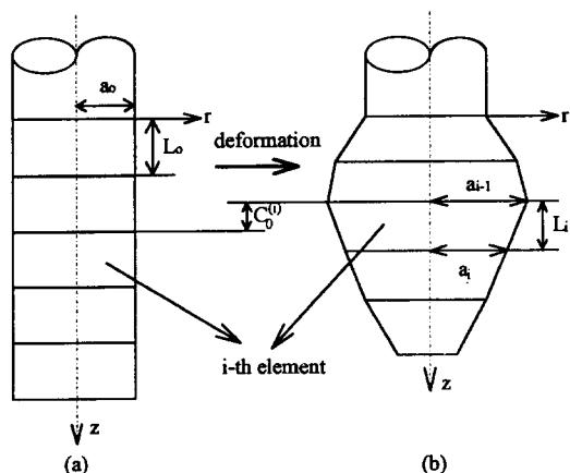
Fig. 1 Discretization of molten tip by slabs
