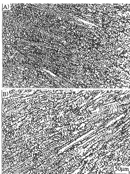
Fig. 3 Microstructures of GTA welds in nitrogen-bearing stainless steels.
