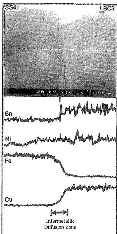
Fig. 6 EDS analysis of interface of the bonded SS41/LBC3 at 850°C for 30 minutes
