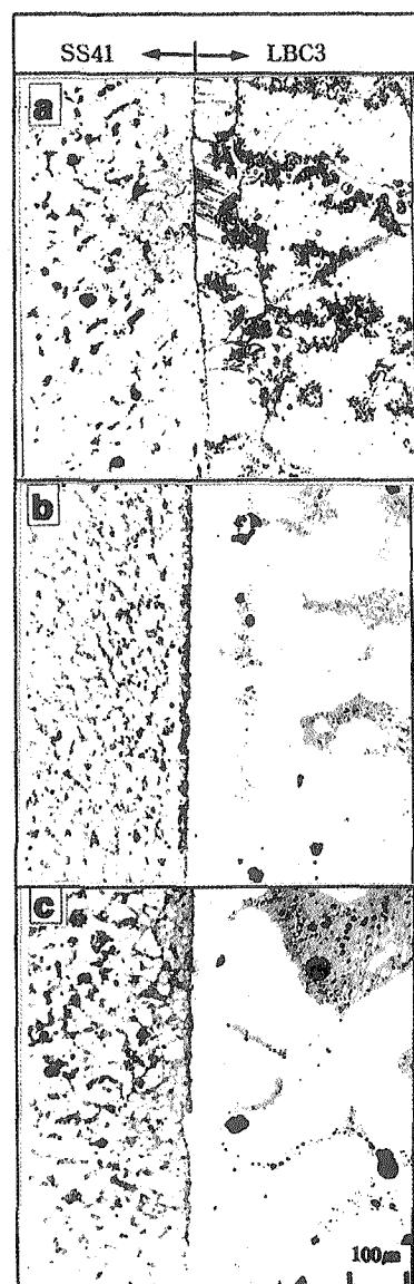
Fig. 5 Optical micrographs of interface of the bonded SS41/LBC3 at 850°C for (a) 10 minutes, (b) 30 minutes and 60 minutes
