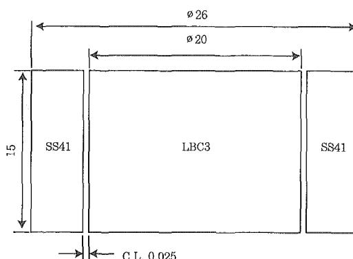
Fig. 1 Schematic drawing of the bonding specimen
