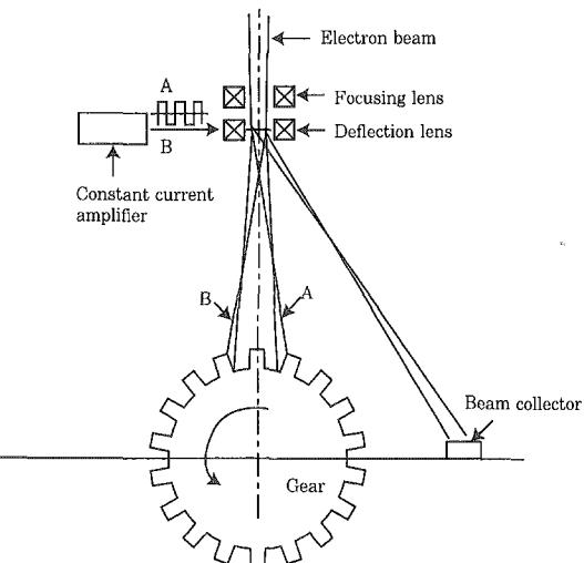
Fig. 12 Quenching method of miniature gear
