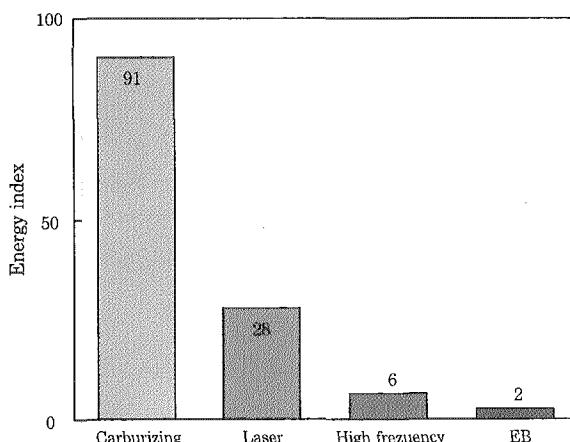
**Fig. 10** Comparison of energy index for quenching methods
