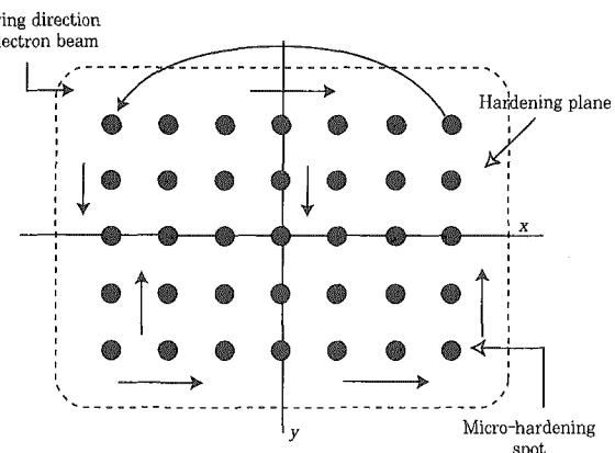
Fig. 8 Micro-dot pattern of the electron beam
