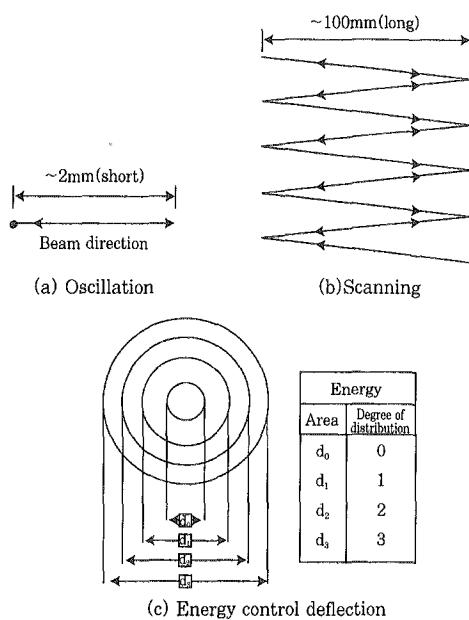
Fig. 3 Typical examples of beam deflection pattern
