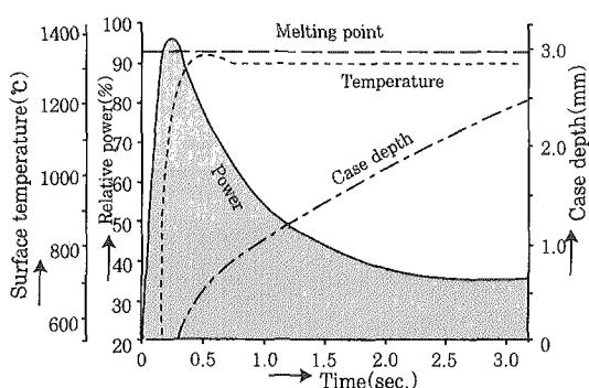
Fig. 7 Typical example of optimal heating pattern
