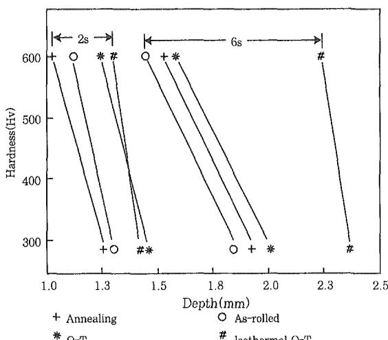
Fig. 9 Effects of hardenability with pre-heat treatment
