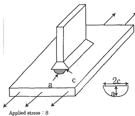
Fig. 4 Semi-elliptical surface crack at weld toe of T-joint
