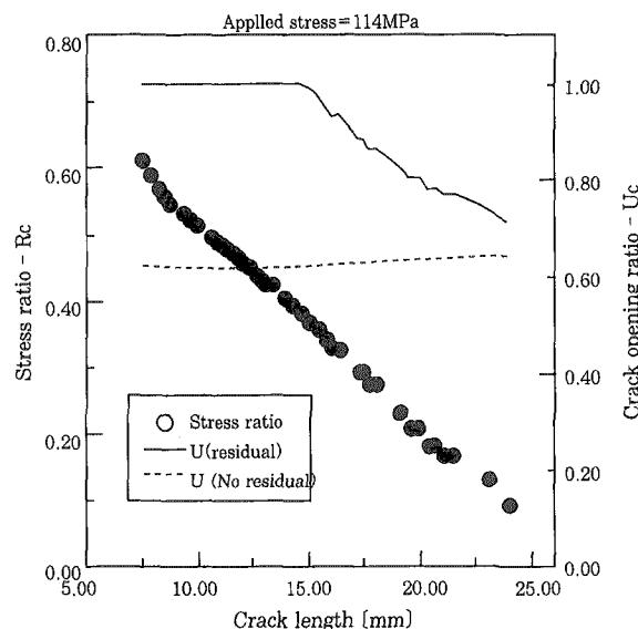
(a) Change of R & U in crack length direction
