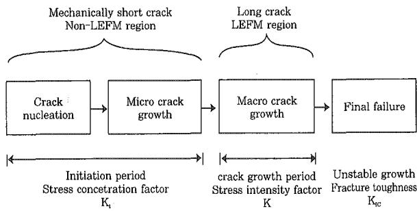
Fig. 1 Classification of fatigue life and its relevant parameter<sup>1)</sup>
