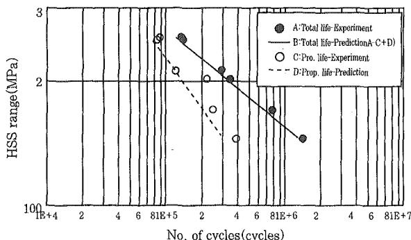
Fig. 15 Propagation and fracture life of hopper knuckle
