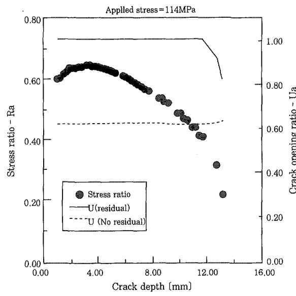
(b) Change of R & U in crack depth direction
