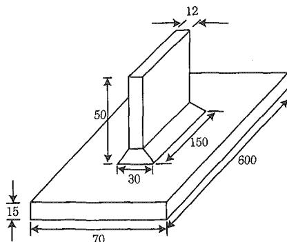
Fig. 8 Detail dimension of T-joint specimen(mm)
