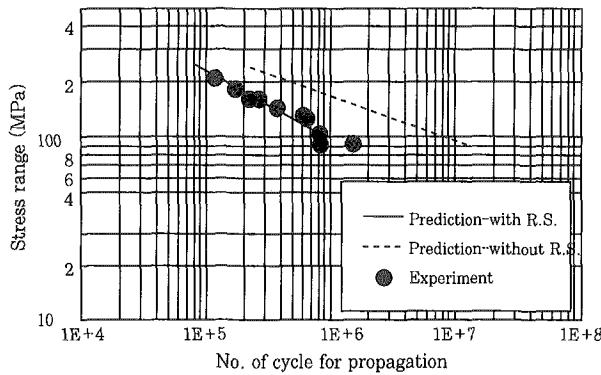
Fig. 12 Effect of residual stress on propagation life
