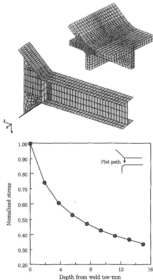
Fig. 14 FE model and stress distribution
