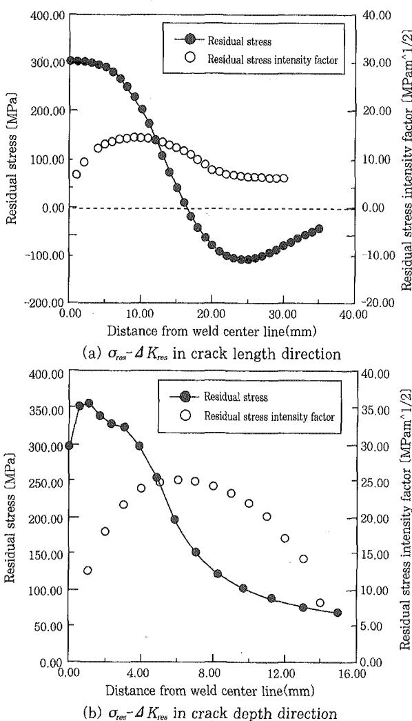
Fig. 6 Residual stress and residual stress intensity factor (T-joint)
