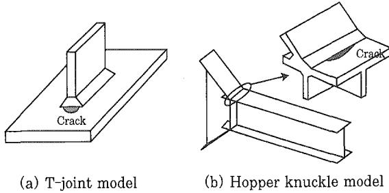
Fig. 2 Schematic view of analysis model
