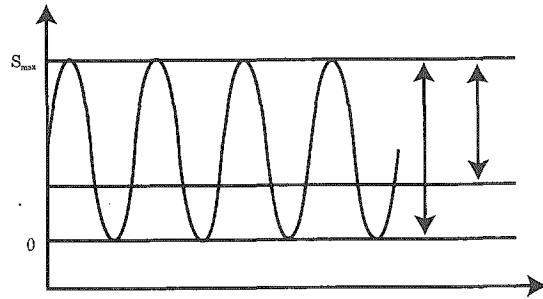
Fig. 3 Crack closure and effective stress intensity factor range
