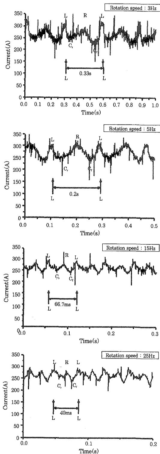
Fig. 5 Current waveform for rotating arc welding
