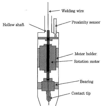
Fig. 2 Schematic diagram of developed electrode nozzle
