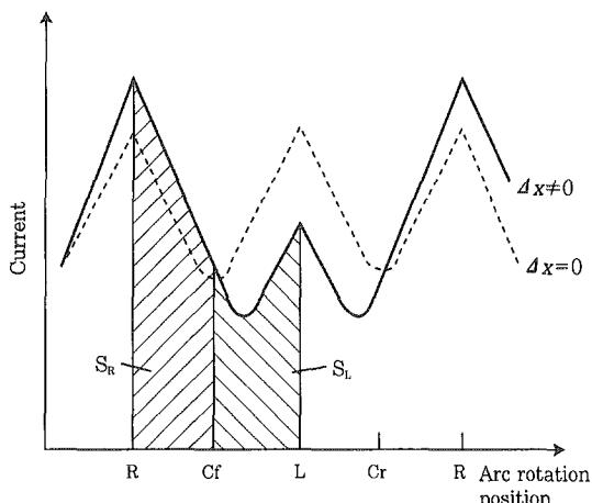
Fig. 7 Typical welding current in rotating arc
