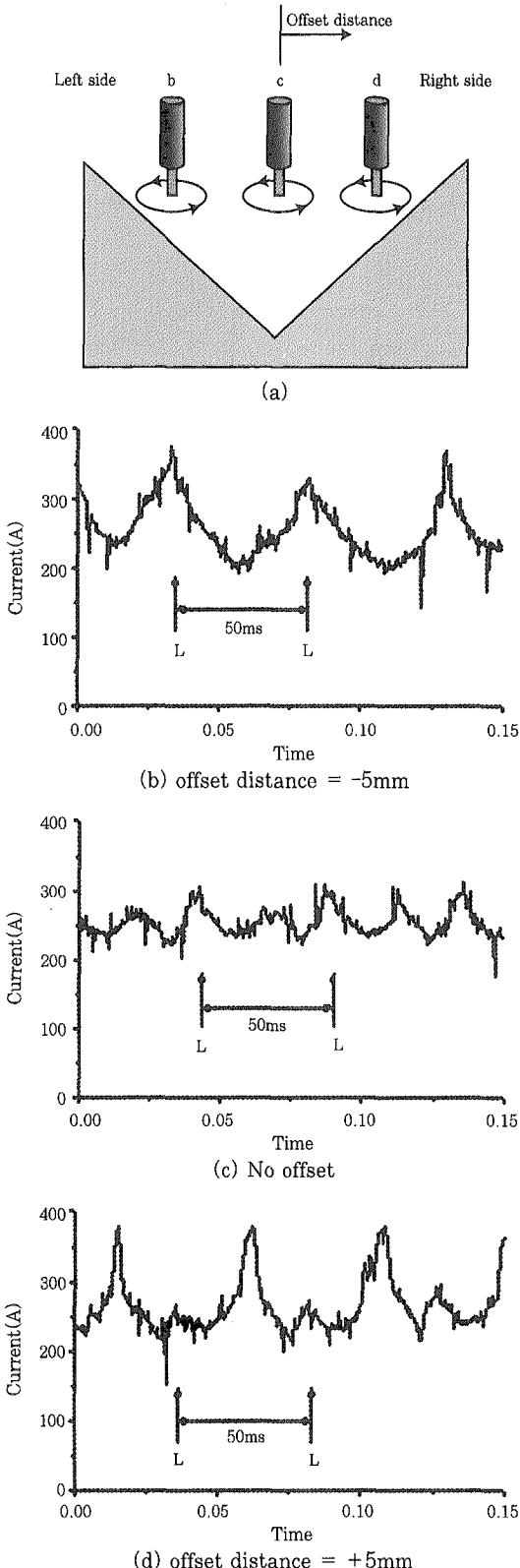
Fig. 8 Welding current signal for various offset
