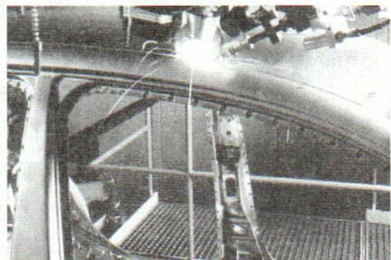
Fig. 3 Roof seam laser welding
