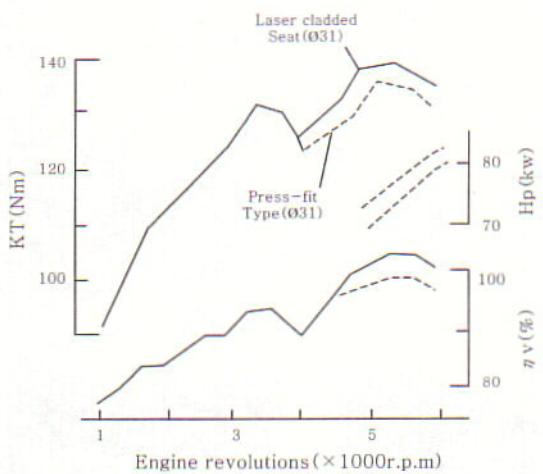
Fig. 5 Size-up effects of the valve seat diameter
