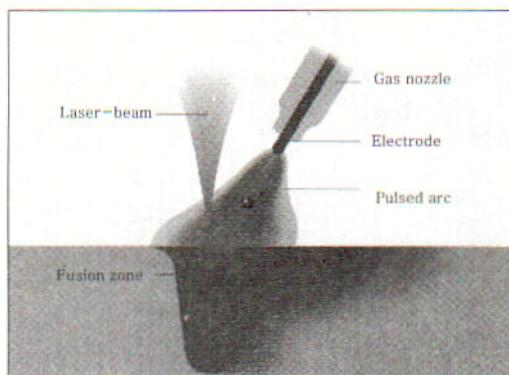
Fig. 7 Schematic diagram of the hybrid welding
