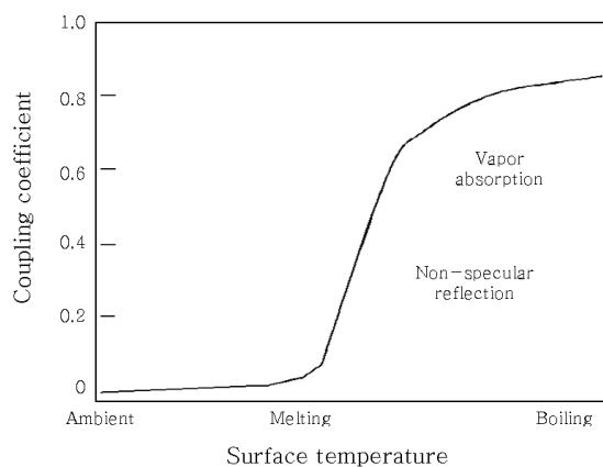
Fig. 2 Coupling coefficient according to material surface temperature
