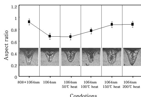
Fig. 5 Transition of aspect ratio for preheating temperature
