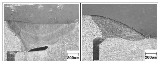
Fig. 11 Cross section of various weld joint by multi-wavelength laser
