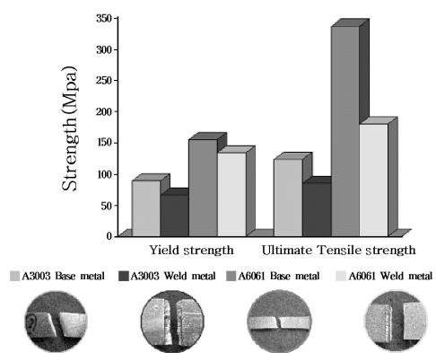
Fig. 14 Tensile strength results
