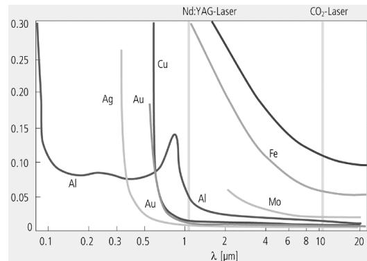
Fig. 1 Absorption of various materials at room temperature
