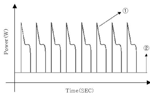
Fig. 4 Output power pattern of hybrid laser beam
