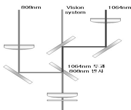
Fig. 3 Configuration of optics
