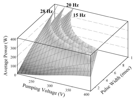
Fig. 1 Plots showing the average output power with the changes of the pumping voltage and pulse width at the pulse frequency of 15, 20 and 28 Hz
