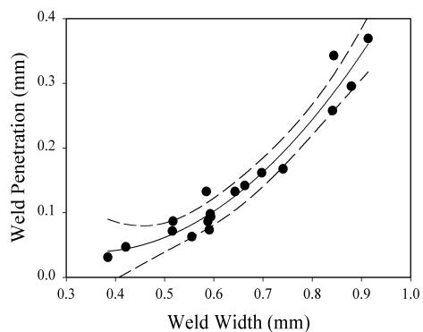
**Fig. 6** Correlation between weld width and weld penetration
