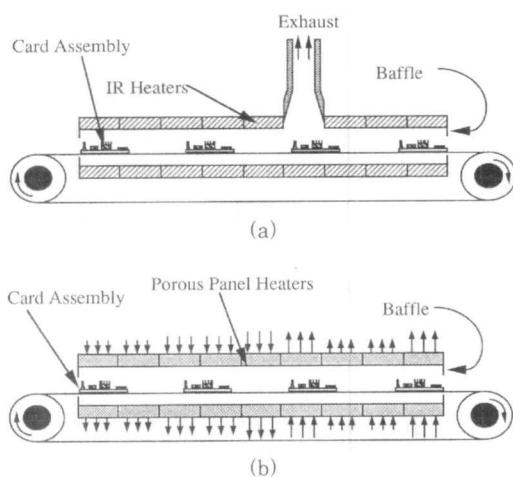
Fig. 1 Schematic of (a) a conventional infrared reflow oven and (b) a forced convection-infrared reflow oven
