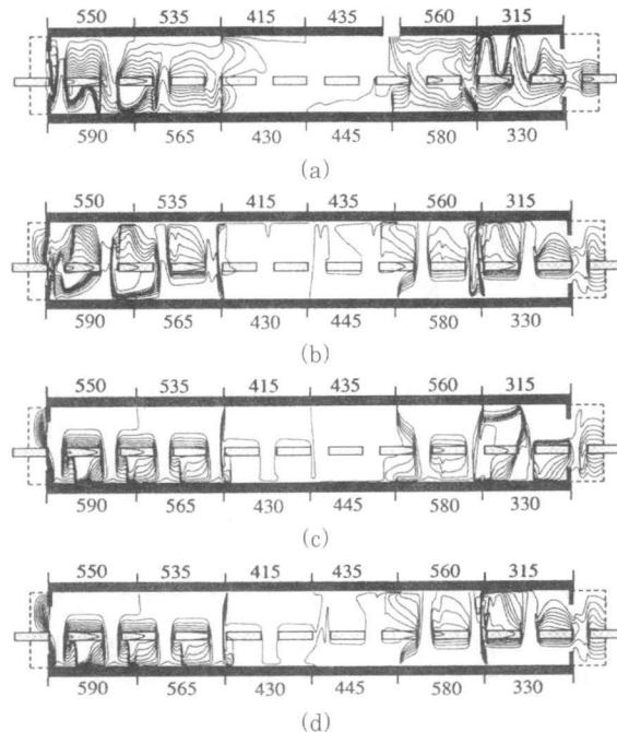
Fig. 3 Predicted temperature distributions within the oven for (a) conventional processing, (b) blowing up, (c) blowing down, and (d) mixed blowing (16 equally-spaced isotherms spanning 300 to 590 K)
