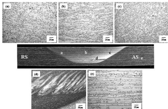
Fig. 4 Each microstructure in the weld of friction stir welded SAF2205: (a) RS (b) Center (c) AS (d) band structure, (e) BM
