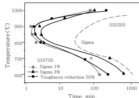
Fig. 2 Isothermal precipitation diagram for S32205 and S32750 duplex stainless steels
