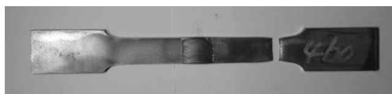
Fig. 9 Fractured tensile specimen of the friction stir welded 2205 duplex stainless steel
