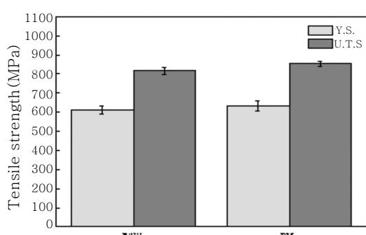
Fig. 10 Tensile properties of the friction stir welded 2205 duplex stainless steel: (a) Y.S. and U.T.S., (b) elongation
