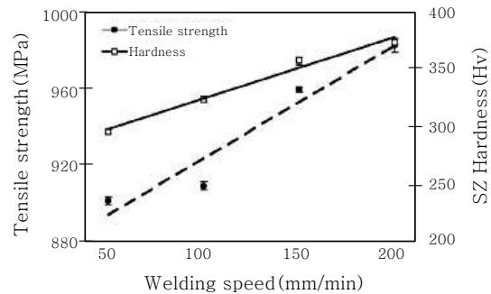
Fig. 11 Effect of FS welding speed on mean hardness value and the tensile strength of the SZ in SAF 2205<sup>23)</sup>
