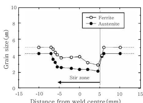
Fig. 6 Grain size profiles of the austenite and ferrite phases in the weld<sup>29)</sup>
