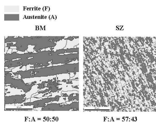
Fig. 8 EBSD map in the weld of friction stir welded SAF2205 : (a) BM, (b) SZ
