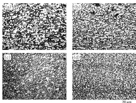
Fig. 7 Optical micrographs showing the grain size in the stir zone at different welding speeds of (a) 50mm/min, (b) 100mm/min, (c) 150mm/min, and (d) 200mm/min<sup>23)</sup>
