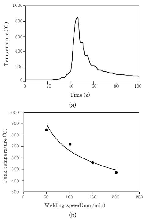
Fig. 1 (a) Thermal profile measured at the welding speed of 50mm/min and (b) Recorded peak temperatures as a function of welding speeds<sup>23)</sup>
