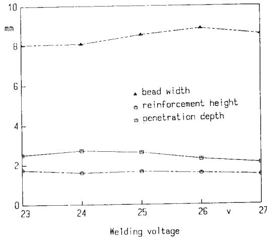
Fig. 7. Weld pool size variation with increasing voltage (4mm thick., wire feed rate: 125 ipm, welding speed: 655 mm/min, peak pulse current: 245A, pulse frequency: 120 pps).
