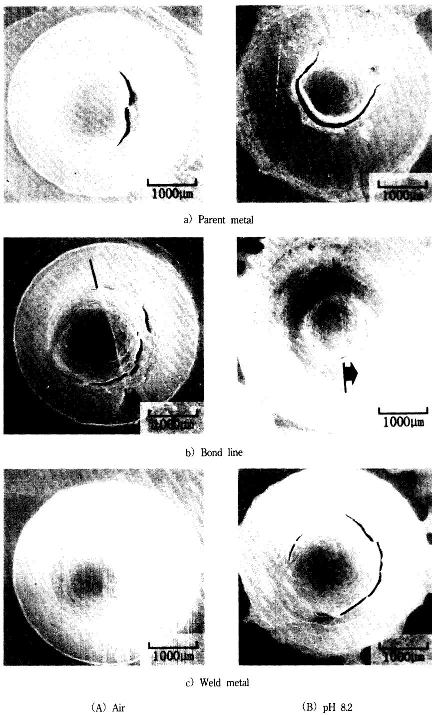
Fig. 8 SEM macrofractographs in HT80 steel-weld joint
