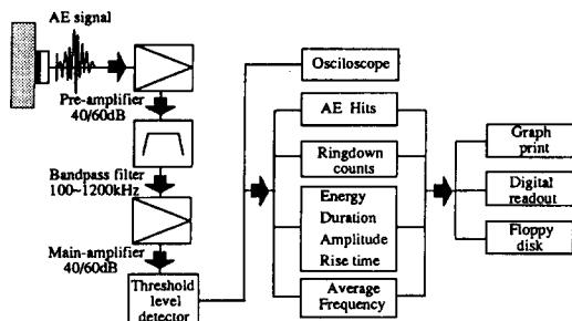
Fig. 4 Block diagram for the AE signal process
