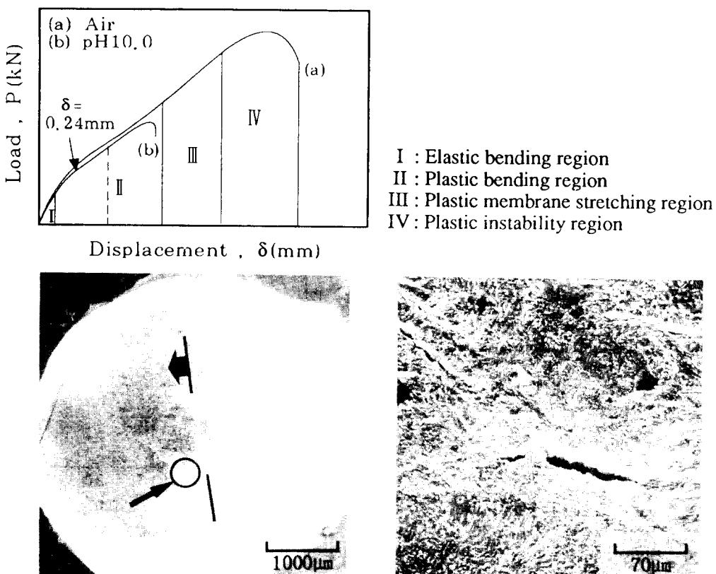
Fig. 12 SEM macro- and microfractographs at = 0.24mm for HT80 steel-bond line in SSW-pH8.2
