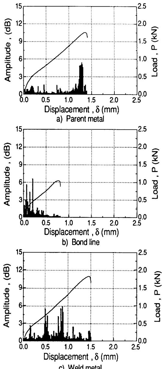
**Fig. 11** AE amplitude distribution plotted along with the load vs displacement for HT80 steel-weld joint in SSW-pH8.2 (Total gain : 80dB, Threshold : 3.55mV)
