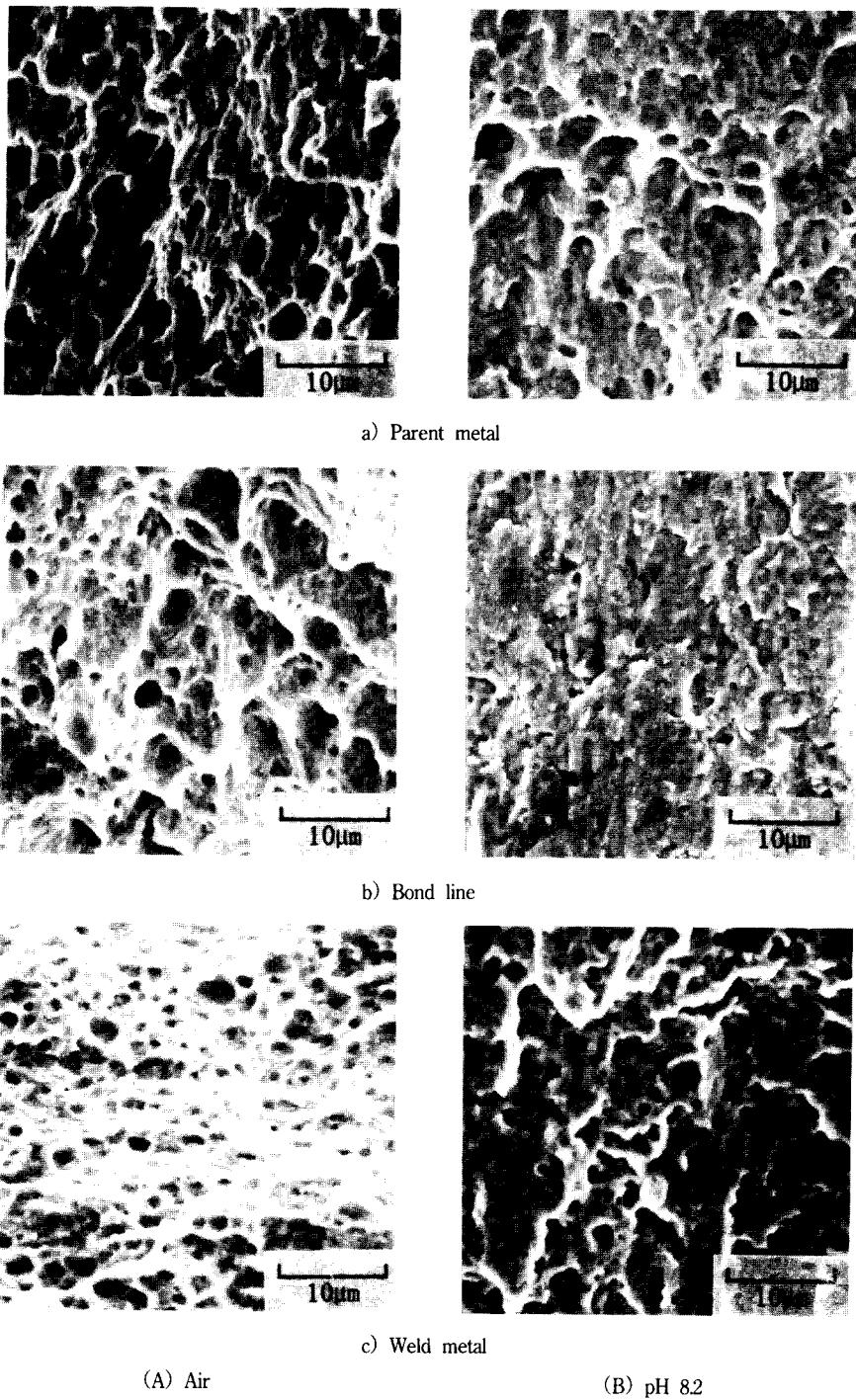
Fig. 9 SEM microfractographs in HT80 steel-weld joint
