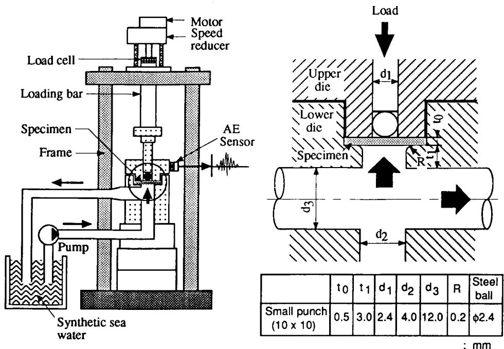
Fig. 3 Schematic illustration of experimental equipments for SP-SSRT
