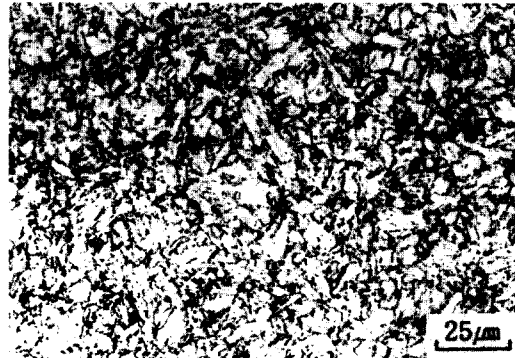
Photo.1 Microstructure of 9% Ni steel
