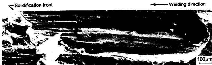
Photo. 3 Microfractograph of solidification crack in DS100 weld metal
