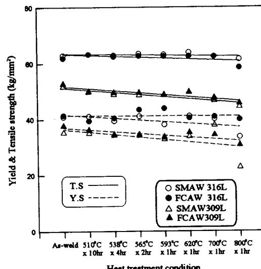
Fig. 2 Effect of PWHT condition on yield &amp; tensile strength in 309L and 316L weldment
