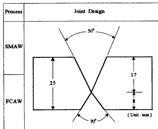
Fig. 1 Groove preparation of the test plate
