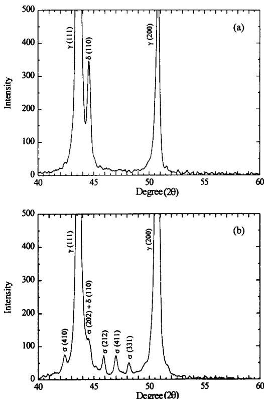
Fig. 5 X-ray diffraction patterns of 309L weld metal
