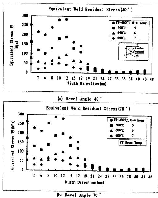
Fig. 6 Distribution of stress Through Width Direction during PWHT (Thickness : 20mm)
