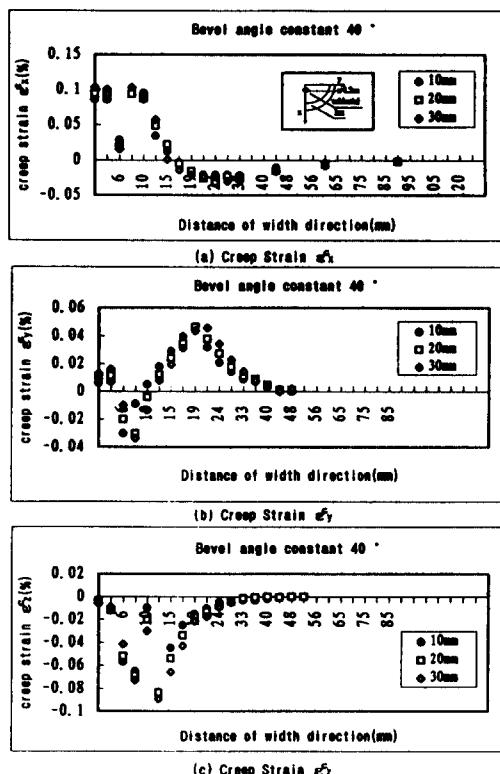
Fig. 3 Distribution of creep strain during PWHT
