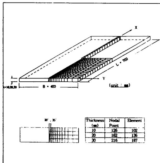
Fig. 1 FEM Model for Welding Residual Stress
