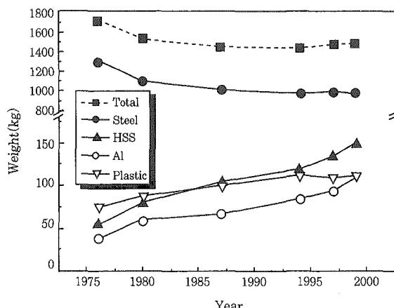
Fig. 1 Weights of materials used in automobile
