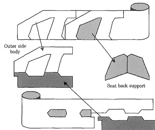
Fig. 4 Nesting of blank components in coil to produce low scrap rate
