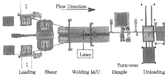
Fig. 1 Lay-out of Laser welding system
