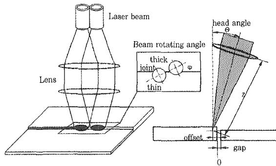
Fig. 2 Dual beam welding
