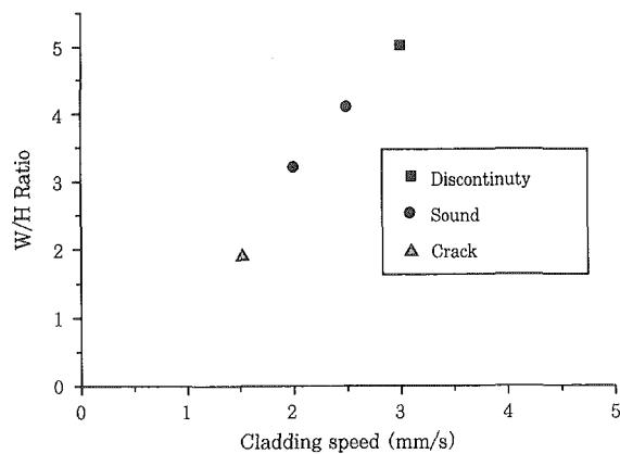
Fig. 4 Relationship between W/H ratio and cladding speed
