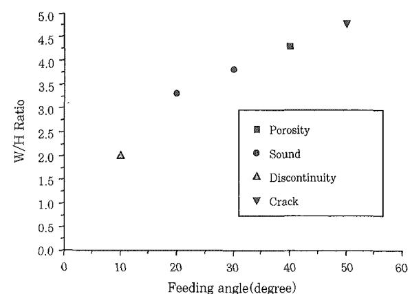
Fig. 3 Relationship between W/H ratio and feeding angle
