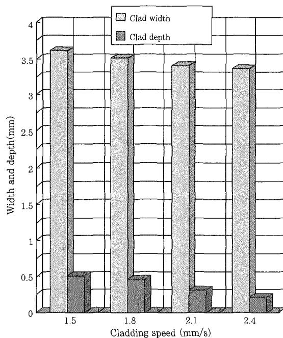
Fig. 7 Width and depth of melt pool at different cladding speed
