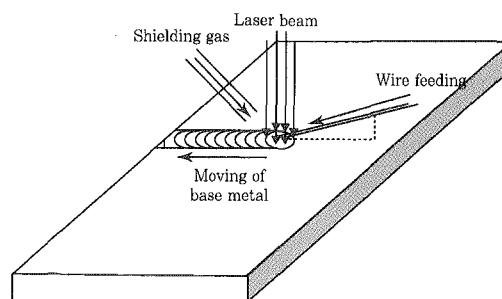
Fig. 2 Wire feeding direction
