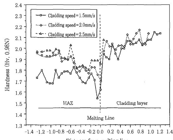
Fig. 10 Hardness distribution of clad layer and HAZ
