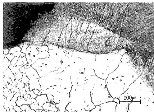
Fig. 9 Boundary between base metal and clad layer
