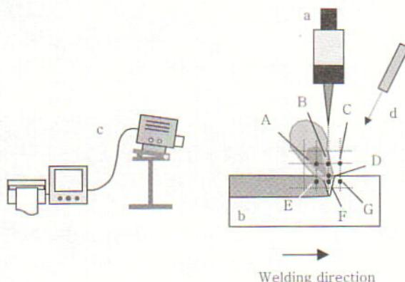
Fig. 1 Test setup for LIP spectrum analysis.
