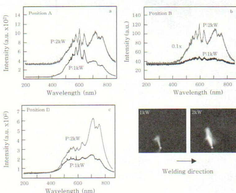
Fig. 3 Effect of applied power on LIP spectra (travel speed: 17mm/s, gas: N<sub>2</sub>)
