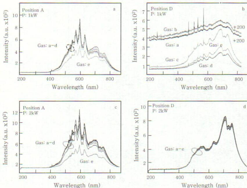
Fig. 5 Effect of assist gas on LIP spectra
