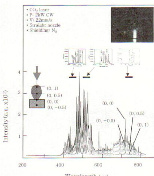
Fig. 4 LIP spectra vs spatial coordinate in the CO<sub>2</sub> laser welding
