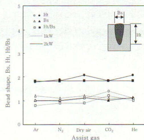
Fig. 6 Effect of assist gas on bead shape
