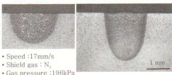
Fig. 8 Bead cross-section
