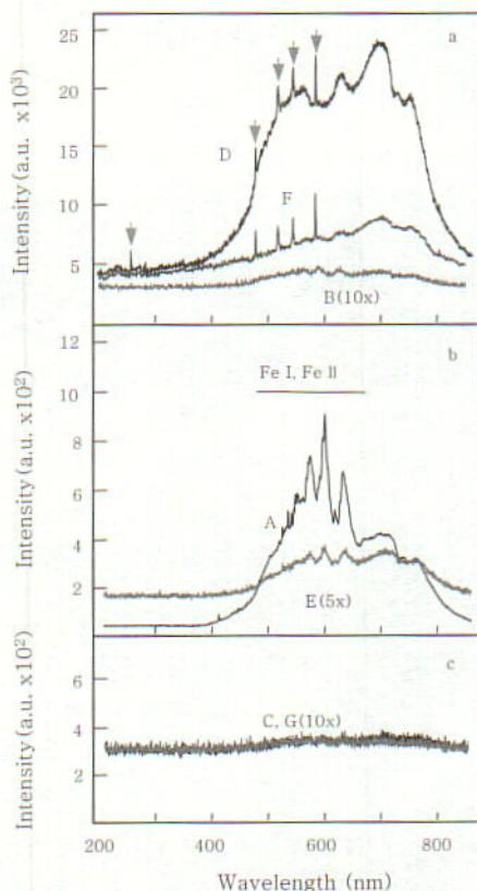
Fig. 2 LIP spectra depending on the spatial coordinate (power: 1kW, travel speed: 17mm/s, gas: N<sub>2</sub>)
