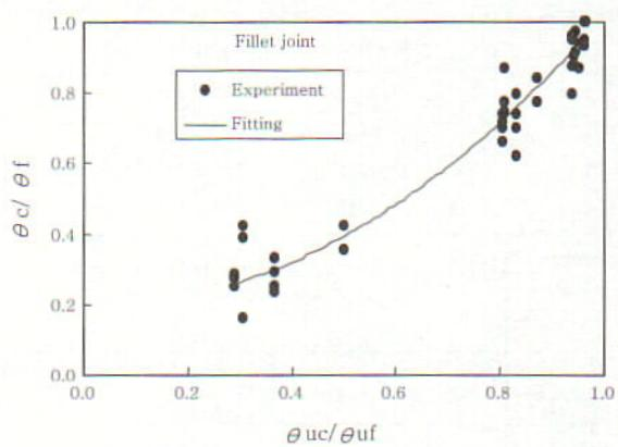
Fig. 12 Constraint coefficient of angular distortion on the fillet welding
