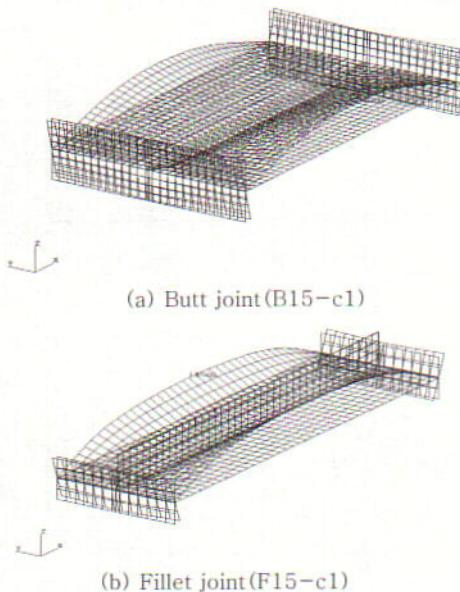
Fig. 9 Deformation shape during unit moment (thickness = 15mm).
