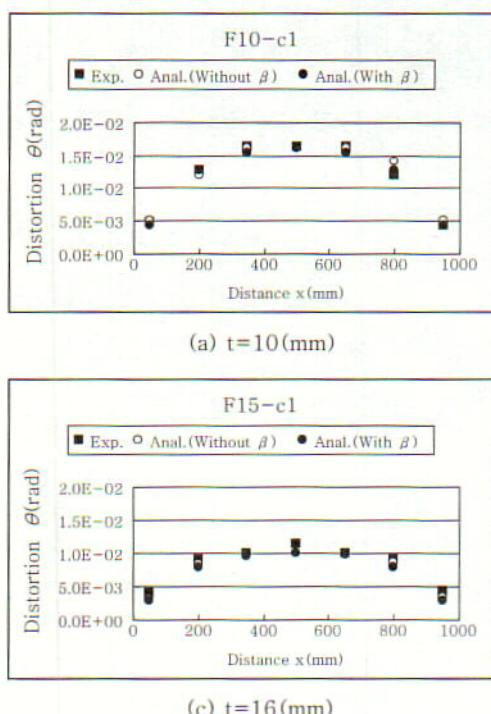
Fig. 17 Angular distortion by fillet welding
