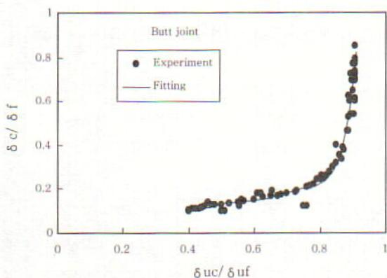
Fig. 10 Constraint coefficient of the transverse shrinkage on the butt welding
