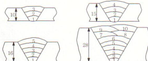
Fig. 4 Deposit sequence by butt welding.
