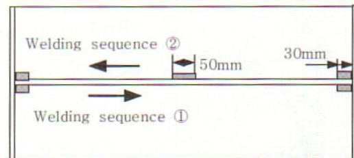
Fig. 5 Location of tack welding and welding sequence
