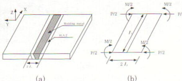
Fig. 1 Mechanical model of welding
