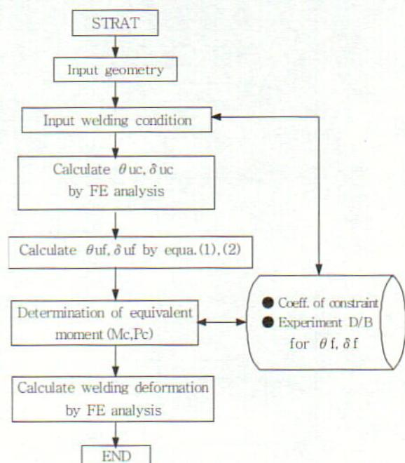
Fig. 14 Flow chart of welding deformation analysis
