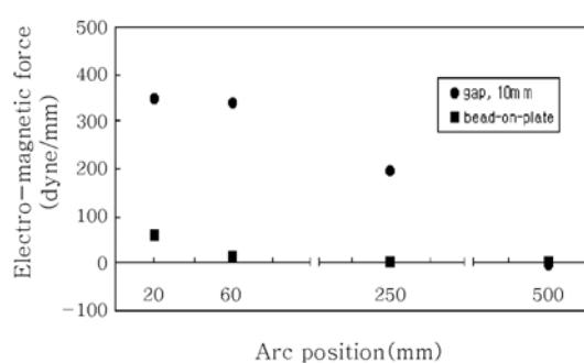
**Fig. 8** Comparison of EMFs at welding start position between in bead-on-plate welding and in butt-joint welding
