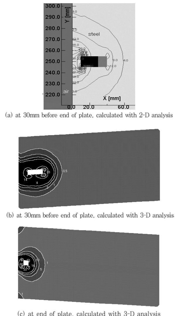
**Fig. 7** Contour of magnetic-flux density with tack weld at end of plate during welding at asymmetric locations
