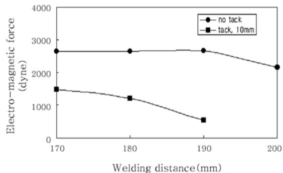
Fig. 6 Effect of tack length at end of plate on electro-magnetic force
