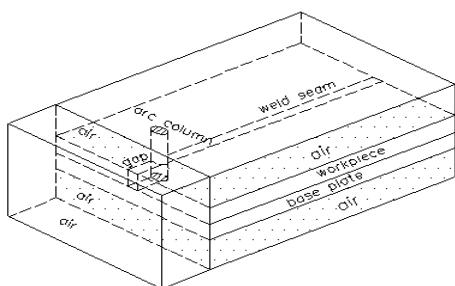
Fig. 2 3-D analysis model with base plate and surrounding air
