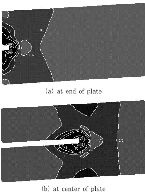
Fig. 5 Contour of magnetic-flux density during welding of butt-joint plate calculated with 3-D analysis
