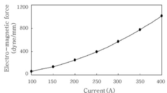
**Fig. 9** Effect of welding current on EMF
