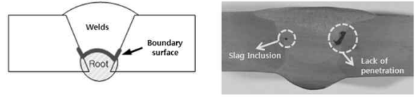
(a) Boundary surface (b) Weld defects Fig. 3 application of 2D weaving patten
