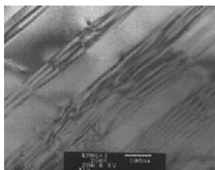
Fig. 4 Strain-induced martensite
