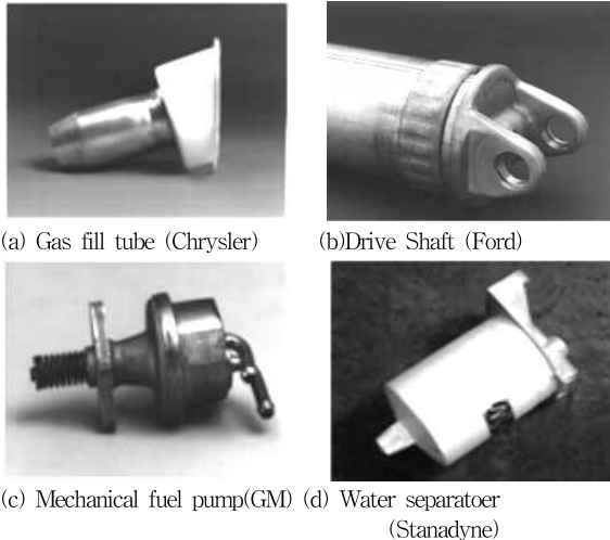
Fig. 3 Manufacture of automotive components using MPW
