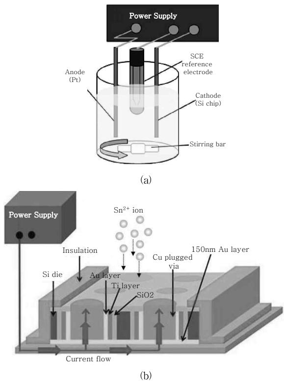
Fig. 5 Schematic diagram of (a) electroplating unit and (b) electroplating Sn bump on the Cu plated via without PR mould
