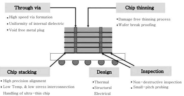
Fig. 1 Technology map of 3-D Stack Packaging<sup>2)</sup>
