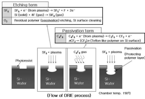
Fig. 2 Schematics of DRIE process
