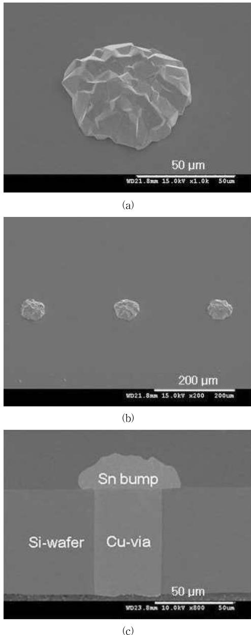
Fig. 6 Sn bumps formed on the Cu filling by DC electroplating without PR mould, (a) bump appearance, (b) bumps having good uniformity, and (c) cross section of a bump<sup>7)</sup>
