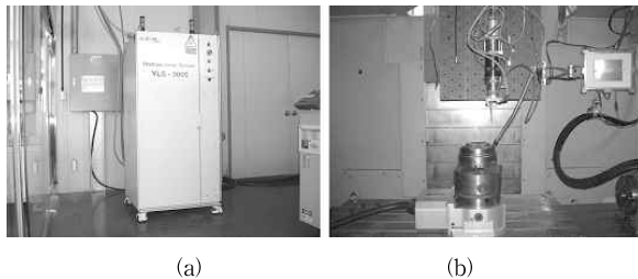
Fig. 2 Experimental apparatus; (a) Fiber laser, (b) Laser welding system
